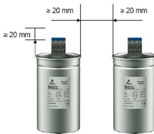
Figure 4: Minimum space over and between the capacitors.
